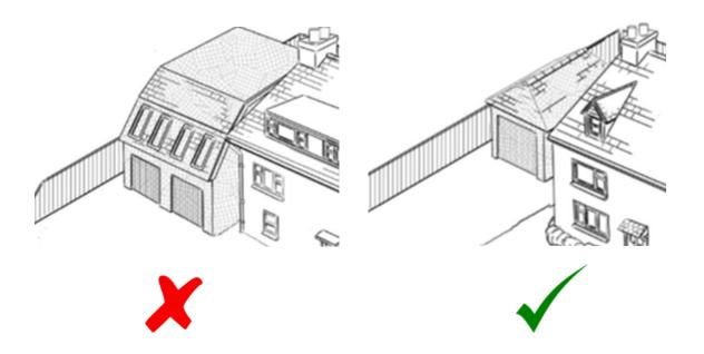
The illustration on the left shows an unacceptable design for a garage, which is set forward of the front main wall and is over-sized relative to the host dwelling.
