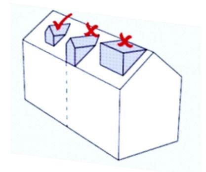
Two of these proposals are unacceptable due to their size, and their intrusive effect on the roof of the existing dwelling. The smaller dormer is in-keeping with the roof of the dwelling and of a more appropriate size.
