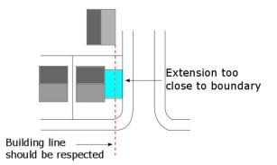
Plan-view of a proposed corner plot extension that is unacceptable because of a failure to respect one of the building lines and because it impinges on the existing boundary.
