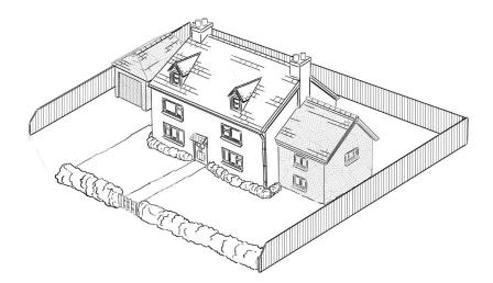
This diagram shows an example of a well thought-out extension and garage, which are subservient to the original house
