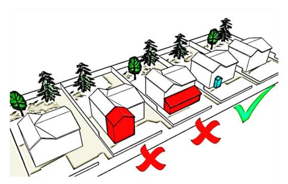
The two proposals in red show front extensions that project significantly from the front wall of the original dwelling, disrupting the building line as a visuallyprominent feature. The third proposal in blue is clearly subservient and does not project far beyond the front wall.
