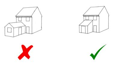
Two versions of a rear extension, showing how the degree of projection can affect the character of the host dwelling. The image on the right hand side illustrates a more sympathetic rear extension.
