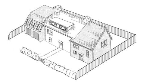
By contrast, this diagram shows an example of poorly-designed extensions that dominate and detract from the original house
