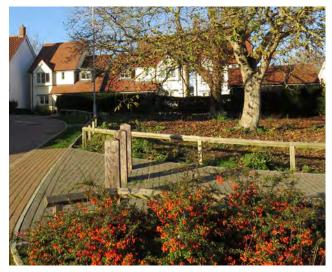
**Figure 85:** Appropriate material change to indicate the footpath/cycle lane within a rural landscape, elsewhere in UK.
