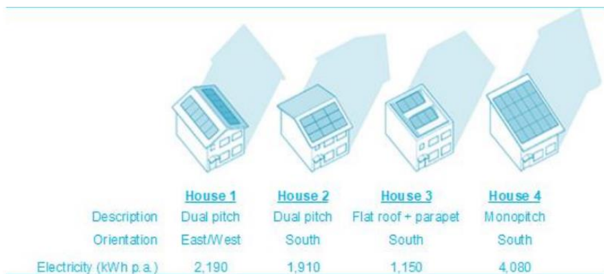
Figure 6. Comparison of electricity generation from PV on houses with different roof shapes. Source: AECOM. 122
